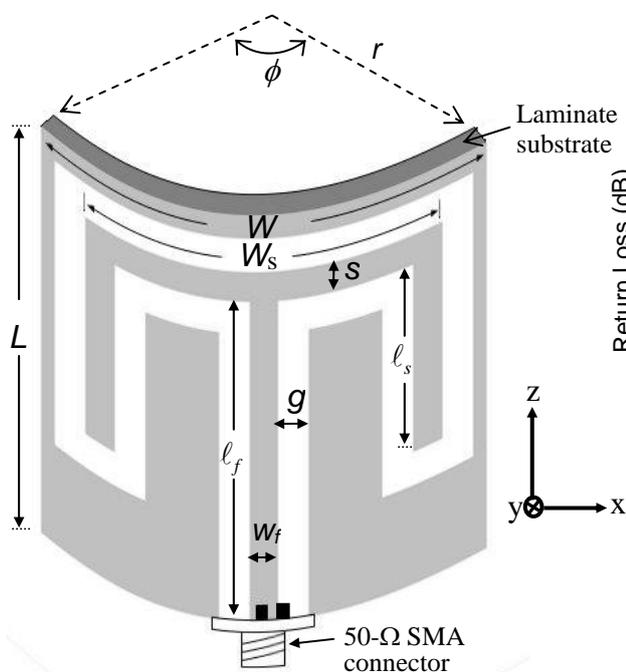
**Figure 1** Configuration of proposed flexible CPW-fed folded-slot monopole antenna for 5.8 GHz tag
