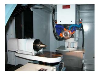
Fig. 9 Five-axis CNC tool grinder
