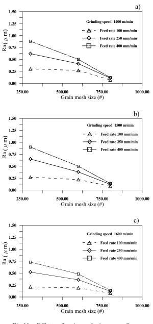
Fig.11 Effects of grain mesh size on surface roughness
