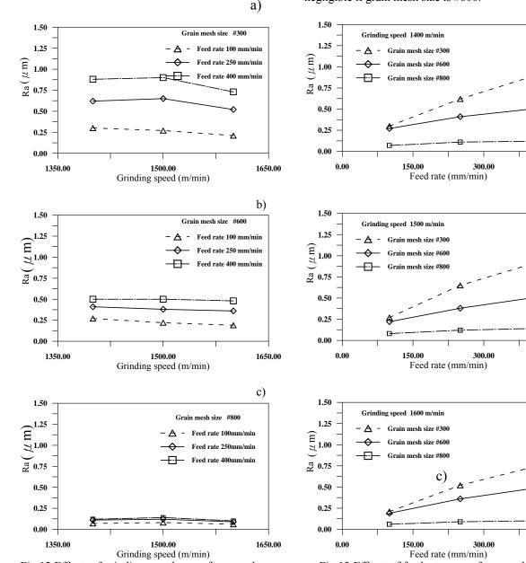
Fig.12 Effects of grinding speed on surface roughness
