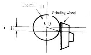
Fig.6 Height difference between the center of the endmill and that of the grinding wheel in grinding of flat relief angle
