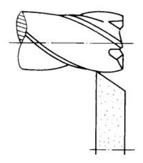
Fig.4 Grinding of concave relief angle using the tip of a grinding wheel
