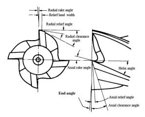
Fig.1 Various angles specified for endmills
