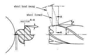
Fig.8 Geometric setting for the eccentric relief angle of the endmill and the grinding wheel
