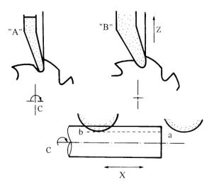
Fig.2 Grinding of radial rake angle
