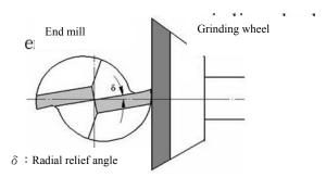
Fig.10 Schematic diagram for grinding of flat relief angle
