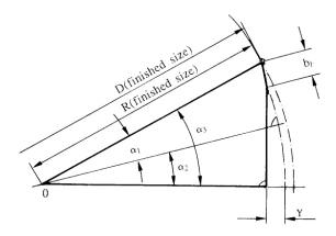
Fig.7 Geometric relation for calculating land of relief plane
