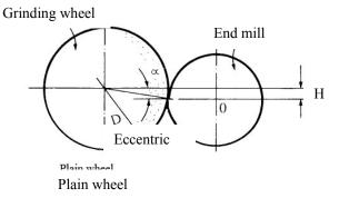
Fig.5 Height difference between the center of the endmill and that of the grinding wheel in grinding of concave relief angle
