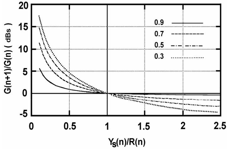
Fig.1  $G(n+1)/G(n)$  Versus  $Y_s / R$  for  $\beta=0.9,0.7,0.5,$  and  $0.3$ .
